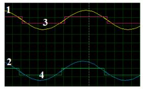
Figure 20. Current phase precedes a voltage of 13.5°. (1 and 3) Wave input current from source; (2 and 4) Wave input voltage from source; (1 and 2) Sine wave input current and voltage to IC LM-324; (3 and 4) Square wave output of IC LM-324 to IC 74LS86
