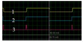
Figure 27. Wave input and output IC 74LS86 at phase angle 4.5°. (1)° Current-phase currents; (2) Square wave phase voltage; (3)°Square wave difference of phase current and voltage
