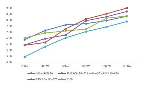
Figure 2. Comparison results of CO2 exhaust emission (in vol%)
