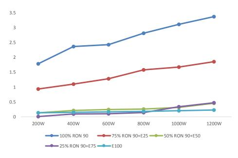
Figure 1. Comparison results of CO exhaust emission (in vol%)
