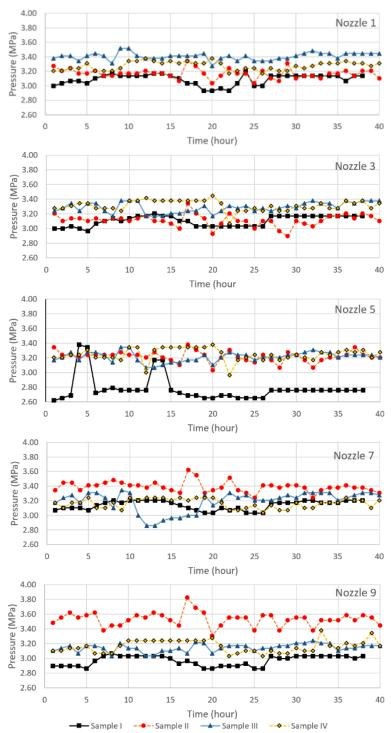
Figure 13. Nozzle pressure profile
