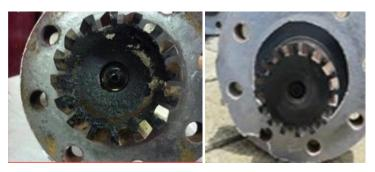
Figure 15. Deposit at No 1 Nozzle, after used Sample I (left side) and Sample III (right side)
