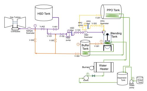
Figure 6. Sub-facilities of blending facility
