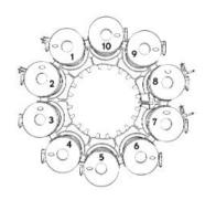
Figure 12. Combustor chambers [6]
