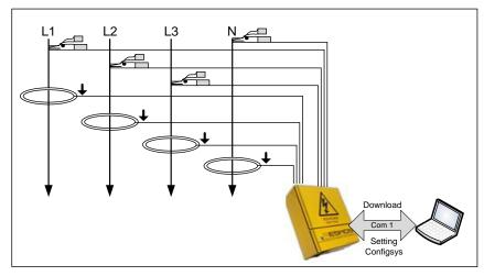
Figure 1. Typical online diagram measurement of a substation network
