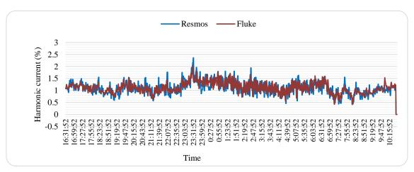
Figure 12. Comparison data IH3Y Resmos and Fluke
