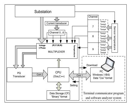
Figure 3. Remote supervising technique communicator
