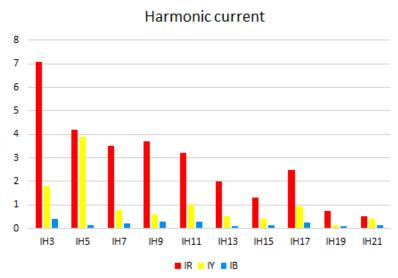
Figure 5. Graphic view on screen harmonic current
