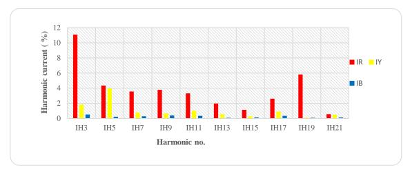
Figure 8. Current harmonic spectrum for residential load
