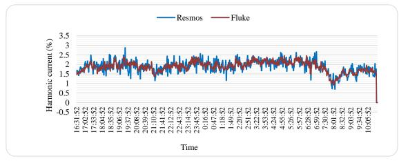
Figure 13. Comparison data IH3B Resmos and Fluke
