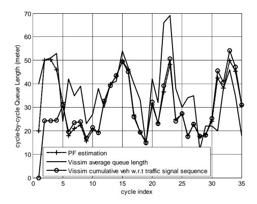
Figure 5. Queue length estimation in VISSIM
