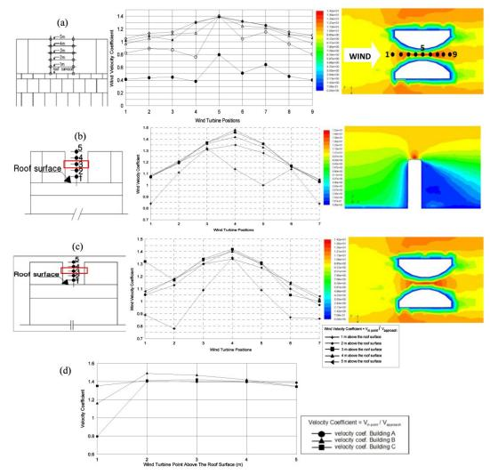
Figure 2. Location of measurement point, wind speed coefficient result and wind speed contour: (a) Building A, (b) Building B, (c) Building C, (d) Wind velocity coefficient comparison between Building A, Building B and Building C. The highest wind velocity coefficient is in Building B
