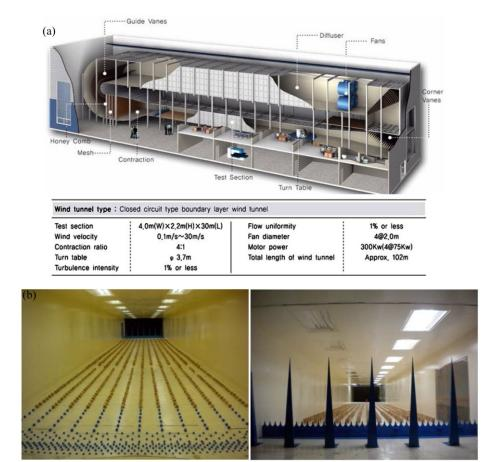
Figure 3. (a) Wind tunnel at CKP wind solutions, South Korea; (b) Roughness block of terrain B in wind tunnel experiment
