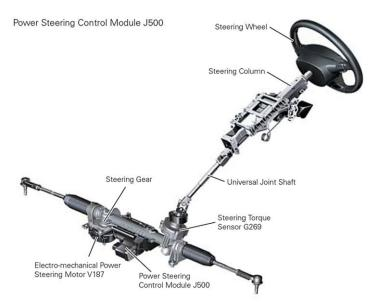
Figure 1. Steering system scheme on the main components that constitute it [2]
