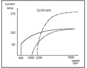
Figure 1. Characteristic of current – speed measured from three car alternators.
