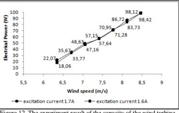
Figure 12. The experiment result of the capacity of the wind turbine.
