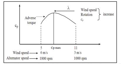
Figure 9. Correlation among wind speed, alternator speed, lambda, and power coefficient.
