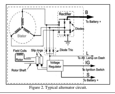
regulator monitors the voltage coming out of the alternator and, when it reaches a threshold of about 14.5 volts, the regulator reduces the excitation current in the rotor to weaken the magnetic field. When the voltage drops below this threshold, the current flows to the rotor is increased.
