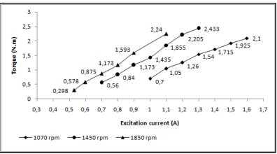
Figure7. Torque vs. excitation current at maximum efficiency.
