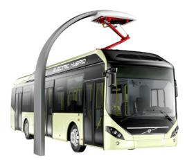
FIGURE 12: City bus Volvo 7900 Electric Hybrid is a combination of an electric bus with a hybrid bus. In the city it can run in pure electric mode and with the recharging of batteries at selected stops; outside the town center it runs in a hybrid mode, whereby the diesel engine is off at the stops, and bus leaves the stop on electric drive only. The diesel engine then starts at a speed of 20 km/h.
