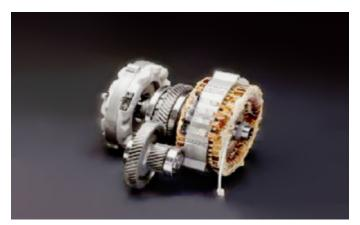
FIGURE 5: Toyota Hybrid Synergy Drive uses a planetary power divider, has no clutch or gear shifting members and continuously varies the gear ratio as a CVT
