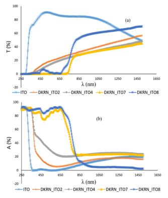
Figure 3: (a) transmittance and (b) absorbance according to the UV-Visible-NIR wavelength for different samples
