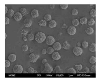
Figure 2. SEM micrograph of the microparticles of CHI/DI-31 obtained by spray drying.
