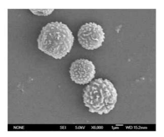
Figure 1. SEM micrograph of the CHI/DI-31 + TPP microparticles obtained by spray driying.
