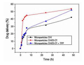
Figure 4. Microparticle release profile in ethanol / water
