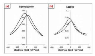
Figure 3: Electrical field dependences of (a) the permittivity and (b) the dielectric losses for the BNT thin film.
