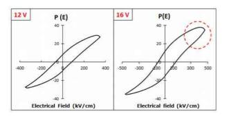
Figure 4: Room temperature macroscopic ferroelectric hysteresis (P-E) loops measured for a BNT film, for an applied voltage of 12 and 16V.
