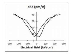
Figure 5: d<sub>33eff</sub> (E) loop of BNT film.
