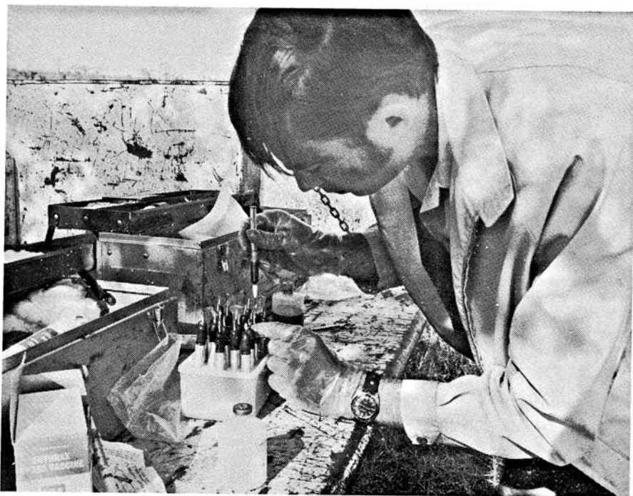
Fig. 2. Stain solution being injected into the receptacle of the marker device.
