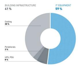
Fig. 2. Energy consumption in the data center building
