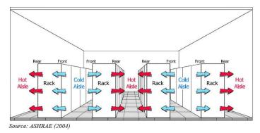
Fig. 5. Typical hot / cold aisle design [13]
