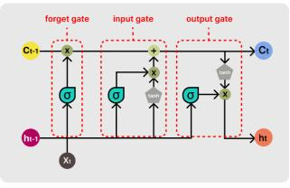
Fig. 5. Memory cell LSTM
