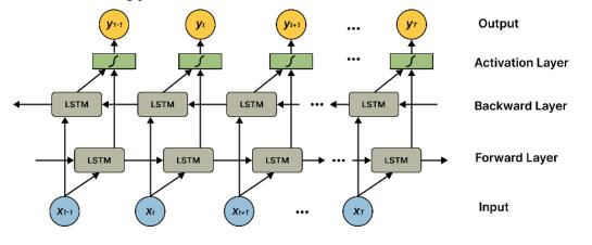
Fig. 6. Bi-LSTM Architecture
