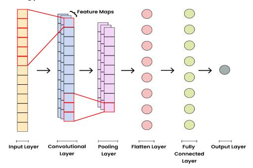
Fig. 3. 1D-CNN architecture
