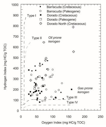
Figure 5: The modified Van Krevelen diagram shows kerogen types in the offshore Mannar Basin (modified after Ratnayake et al., 2018a).
