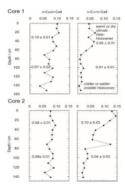
Figure 7: The distribution of n-C<sub>29</sub>/n-C<sub>all</sub> and n-C<sub>37</sub>/n-C<sub>all</sub> ratios in Bolgoda Lake sediments (modified after Ratnayake et al., 2017b).
