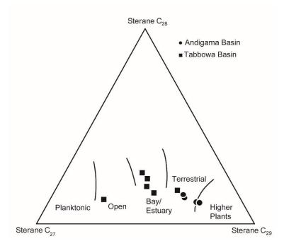
Figure 3: Comparison of OM sources and depositional environments of the Andigama and Tabbowa Basins using the ternary diagram of  $C_{27}$ - $C_{28}$ - $C_{29}$ steranes (modified after Huang and Meinschein, 1979; Ratnayake and Sampei, 2015).
