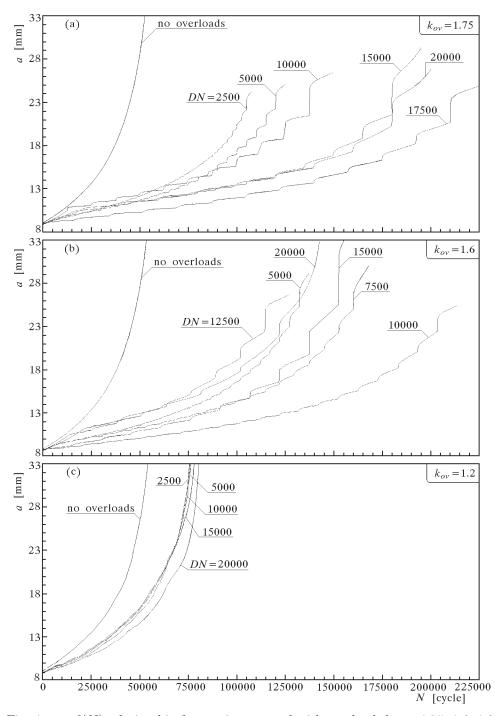
Fig. 4. a = f(N) relationship for specimen tested with overload  $k_{ov} = 1.75, 1.6, 1.2$
