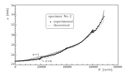
Fig. 3. Theoretical description of crack propagation in CT specimens made of 18G2A steel
