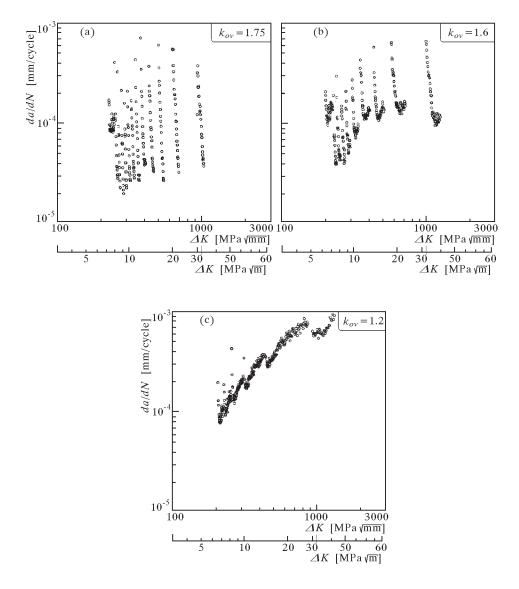
Fig. 5.  $da/dN = f(\Delta K)$  relationship for specimen tested with overload  $k_{ov} = 1.75$ , 1.6, 1.2
