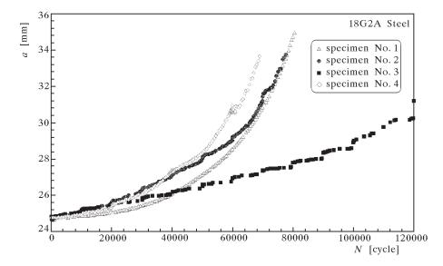
Fig. 2. Crack length a vs. number of cycles N for CT specimens made of 18G2A steel under fatigue tests with overloads applied in cycles
