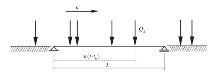
Fig. 1. The beam loaded by a random train of forces travelling in the same direction, all with equal, constant velocities u
