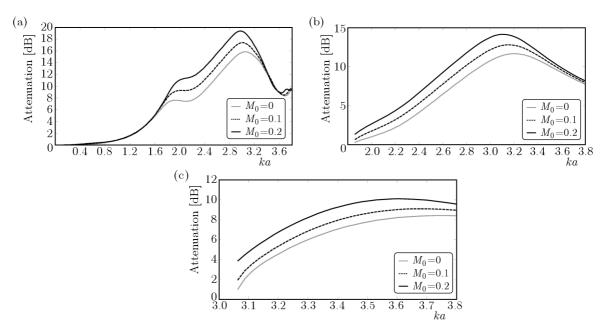
Fig. 4. Acoustic power attenuation of the studied duct in the presence of (0,0) mode (a), (1,0) mode (b) and (2,0) mode (c) versus ka for several Mach numbers
