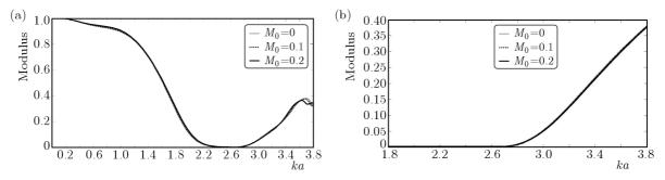
Fig. 2. Modulus of the transmission coefficients  $T^+_{00,00}$  (a) and  $T^+_{10,10}$  (b) versus ka for several Mach numbers
