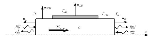
Fig. 1. Schematic of the theoretical model for the computation of the multimodal scattering matrix
