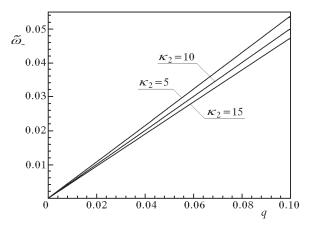
Fig. 4. Diagrams of spectral lines for lower frequencies in the finite difference models and the first and second order continuum models
