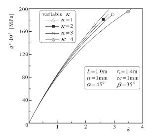
Fig. 5. Equilibrium paths; pressure q versus deflection  $\widetilde{w}$
