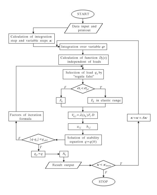
Fig. 4. Simplified block diagram of the algorithm for numerical calculation
