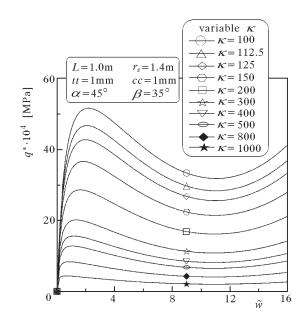
Fig. 6. Equilibrium paths; pressure q versus deflection  $\widetilde{w}$
