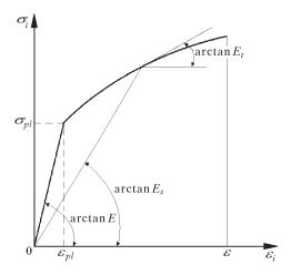
Fig. 3. Nonlinear stress-strain relation
