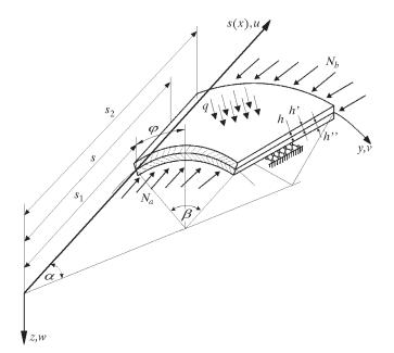
Fig. 1. Subject of consideration – bilayered open conical shell
