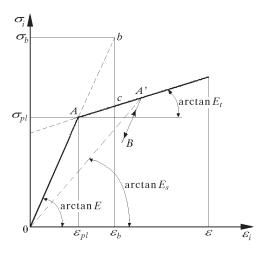
Fig. 2. Bilinear stress-strain relation
