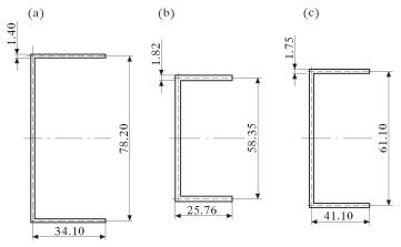
Fig. 3. Optimal profiles of channels with the same area  $(Q^* = 0.2)$  for L = 1 m: (a) steel; (b) composite A; (c) composite B
