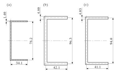
Fig. 4. Optimal profiles of channels with the same weight  $(Q^* = 0.2)$  for L = 1 m: (a) steel; (b) composite A; (c) composite B
