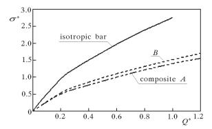
Fig. 8. Nondimensional critical stresses  $\sigma^*$  versus  $Q^*$  for the isotropic and composite materials
