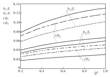
Fig. 5. Cross-sectional nondimensional parameters  $b_1/L$ ,  $b_2/L$ ,  $t/b_1$ ,  $t/b_2$  versus  $Q^*$  for composite A (broken line) and for the isotropic material (full line)
