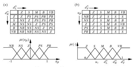
Fig. 3. Angular (a) and linear (b) velocity coefficient rules, respectivly
