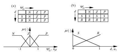
Fig. 5. Angular (a) and linear (b) velocity coefficient rules
