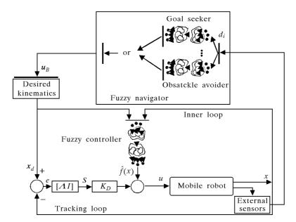
Fig. 2. Navigator and controller
