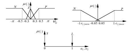
Fig. 12. Membership functions of corresponding to the fuzzy terms presented in Fig. 13  $$\rm Fig.\,13$$
