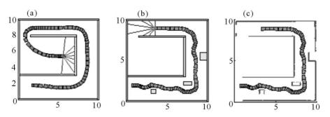
Fig. 4. Reaching the middle of a collision-free space behaviour
