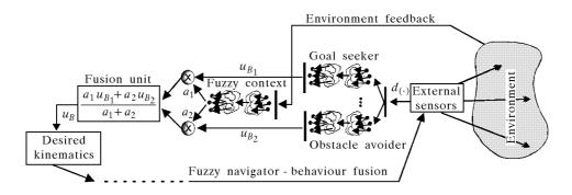
Fig. 10. Basic structure of the fuzzy navigator
