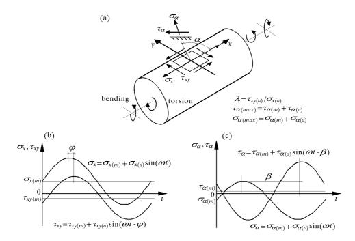
Fig. 1. Non-proportional stress histories; (a) definition of the directions x and  $\alpha$ , (b) stress histories in the direction x, (c) stress histories in the direction  $\alpha$
