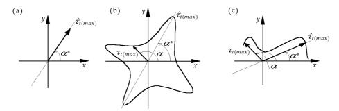
Fig. 2. The distinguished states of the maximum shear stress vector; (a)  $\varphi = 0$ ,  $\sigma_{x(m)} = \tau_{xy(m)} = 0$ , (b)  $\varphi \neq 0$ ,  $\sigma_{x(m)} = \tau_{xy(m)} = 0$ , (c)  $\sigma_{x(m)} \neq 0$ ,  $\tau_{xy(m)} \neq 0$
