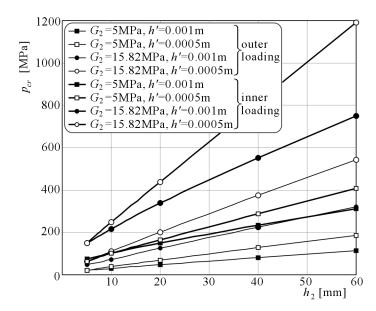
Fig. 5. Critical static load distributions depending on core thickness for plates compressed on the inner and outer perimeter
