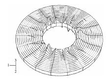
Fig. 11. Critical buckling form of the plate with parameters: h' = 0.0005 m,  $h_2 = 0.06 \text{ m}$  and  $G_2 = 15.82 \text{ MPa}$ , loaded on outer perimeter
