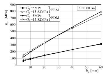
Fig. 17. Critical load distribution depending on the core for the plate with equal layer deflections, loaded on the inner perimeter and with facing thickness  $h' = 0.001 \,\mathrm{m}$
