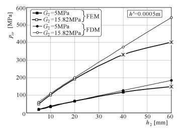
Fig. 7. Critical static load distribution depending on the core for the plate loaded on the outer perimeter with facing thickness  $h' = 0.0005 \,\mathrm{m}$
