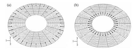
Fig. 2. Scheme of the plate loaded: (a) on the outer perimeter, (b) on the inner perimeter
