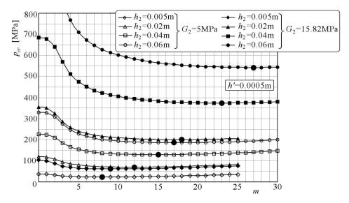
Fig. 3. Critical static load distributions depending on the number of buckling waves for the plate compressed on the outer perimeter with facing thickness  $h' = 0.0005 \,\mathrm{m}$
