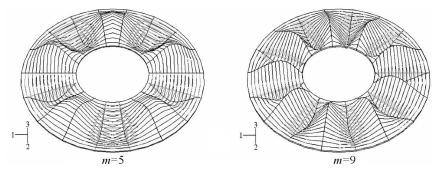
Fig. 13. Exemplary critical buckling forms of plates loaded on the outer perimeters
