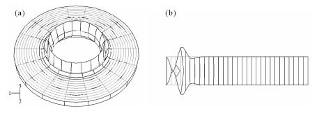
Fig. 12. Critical buckling form of the plate with parameters: h' = 0.0005 m,  $h_2 = 0.06 \text{ m}$  and  $G_2 = 15.82 \text{ MPa}$ , loaded on inner perimeter and built: (a) as full annulus, (b) of axisymmetric elements
