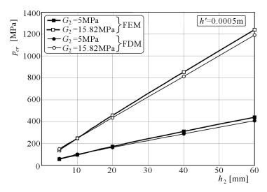
Fig. 16. Critical load distribution depending on the core for the plate with equal layer deflections, loaded on the inner perimeter and with facing thickness  $h' = 0.0005 \,\mathrm{m}$
