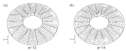
Fig. 18. Critical buckling form of the plate loaded on the outer perimeter with equal layer deflections and with parameters h' = 0.0005 m,  $h_2 = 0.06 \text{ m}$ : (a)  $G_2 = 5 \text{ MPa}$ , (b)  $G_2 = 15.82 \text{ MPa}$
