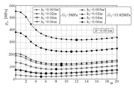
Fig. 4. Critical static load distributions depending on the number of buckling waves for the plate compressed on the outer perimeter with facing thickness h' = 0.001 m
