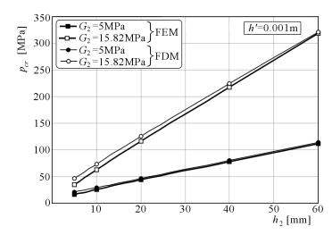
Fig. 15. Critical load distribution depending on the core for the plate with equal layer deflections, loaded on the outer perimeter and with facing thickness  $h' = 0.001 \,\mathrm{m}$
