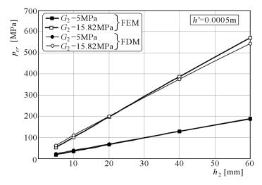
Fig. 14. Critical load distribution depending on the core for the plate with equal layer deflections, loaded on the outer perimeter and with facing thickness  $h' = 0.0005 \,\mathrm{m}$
