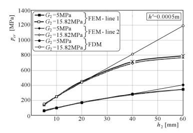
Fig. 9. Critical static load distribution depending on the core for the plate loaded on the inner perimeter with facing thickness  $h' = 0.0005 \,\mathrm{m}$
