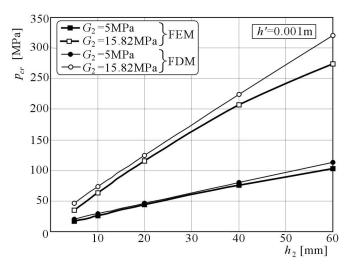
Fig. 8. Critical static load distribution depending on the core for the plate loaded on the outer perimeter with facing thickness  $h' = 0.001 \,\mathrm{m}$
