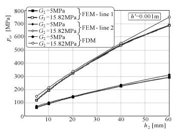
Fig. 10. Critical static load distribution depending on the core for the plate loaded on the inner perimeter with facing thickness  $h' = 0.001 \,\mathrm{m}$
