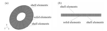
Fig. 6. The scheme of plate mesh: (a) annulus model, (b) model built of axisymmetric elements
