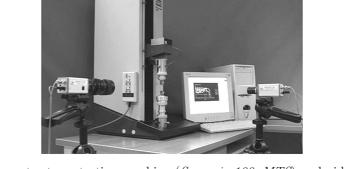
Fig. 1. Measurement set-up: testing machine (Synergie 100, MTS) and videoextensometer (ME 46-350, Messphysik)
