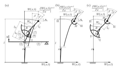
Fig. 4. Deflected form of column type A (see Fig. 2a), geometry and externalisation of internal forces
