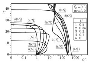
Fig. 13. Curves on the plane: loading parameter – parameter of natural vibration frequency of columns for various parameters  $l_C^*$
