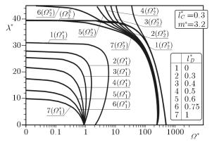
Fig. 11. Curves on the plane: loading parameter – parameter of natural vibration frequency of column  ${\bf A}$
