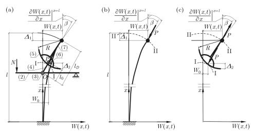
Fig. 5. Deflected form of column **B** (see Fig. 2b), geometry and externalisation of internal forces
