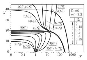
Fig. 12. Curves on the plane: loading parameter – parameter of natural vibration frequency of column  $\mathbf{B}$
