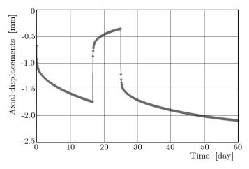
Fig. 4. Axial displacement in viscoelastic panel versus time
