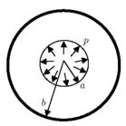
Fig. 5. Viscoelastic cylinder submitted to internal pressure
