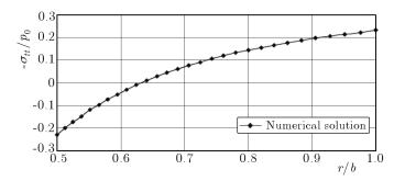
Fig. 8. Variation of the distribution of circumferential compressive stress
