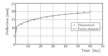
Fig. 2. Deflection in viscoelastic panel versus time
