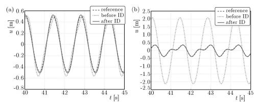
Fig. 9. Case 5. Time history at different degrees of freedom; (a) DOF 2 – not control point, (b) DOF 11 – control point
