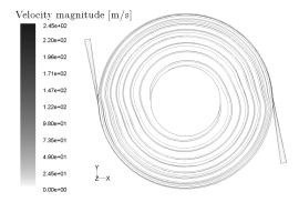
Fig. 11. Pathlines coloured by velocity magnitude; 2 supply nozzles, disk diameter 300 mm, inlet angle 10°; rotational speed 9000 rpm
