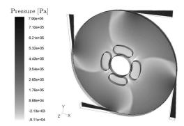
Fig. 13. Full model calculations. Contours of static pressure in the symmetry plane between the disks
