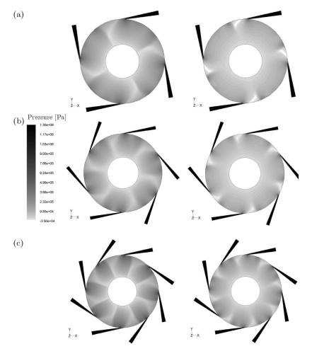
Fig. 5. Contours of static pressure at nominal load, plane of symmetry; four, six and eight nozzle supply, disk diameter 100 mm, inlet angle 10°; (a) 18 000 rpm, (b) 9000 rpm
