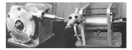
Fig. 2. 4.5" Tesla microturbines working on a water steam
