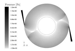
Fig. 9. Contours of static pressure; 2 supply nozzles, disk diameter  $300\,\mathrm{mm}$ , inlet angle  $10^\circ$ ; rotational speed  $9\,000\,\mathrm{rpm}$
