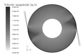
Fig. 10. Contours of velocity magnitude; 2 supply nozzles, disk diameter 300 mm, inlet angle 10°; rotational speed 9 000 rpm
