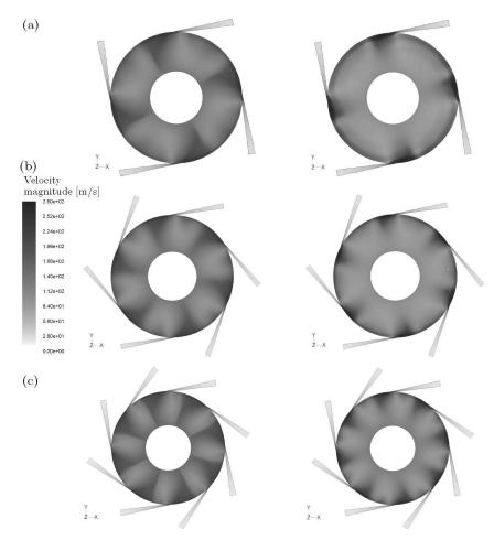
Fig. 6. Contours of velocity magnitude at nominal load, plane of symmetry; four, six or eight supply nozzles, disk diameter  $100 \,\mathrm{mm}$ , inlet angle  $10^\circ$ ; (a)  $18\,000 \,\mathrm{rpm}$ , (b)  $9\,000 \,\mathrm{rpm}$
