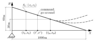
Fig. 2. Final phase of aircraft approach
