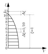
Fig. 2. Discretization of the half-column
