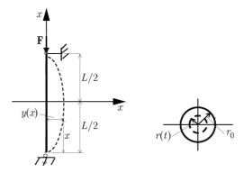
Fig. 1. Bar under axial compressive load P
