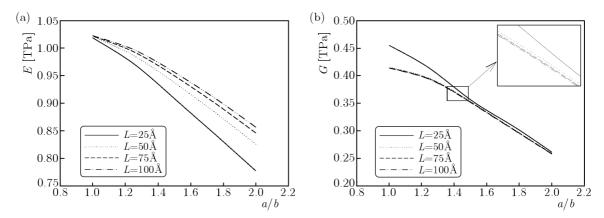
Fig. 9. Variation of Young's modulus (a) and shear modulus (b) of (10,0) with the cross sectional aspect ratio (a/b) for different lengths
