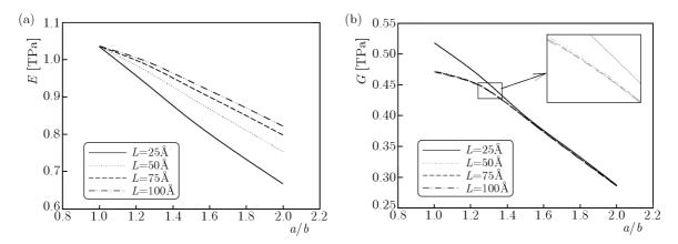
Fig. 11. Variation of Young's modulus (a) and shear modulus (b) of (20,0) with the cross sectional aspect ratio (a/b) for different lengths
