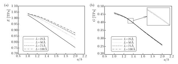
Fig. 5. Variation of Young's modulus (a) and shear modulus (b) of (10, 10) with the cross sectional aspect ratio (a/b) for different lengths
