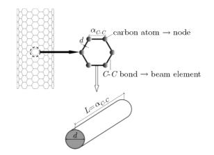
Fig. 1. Simulation of a SWCNT as a space-frame structure
