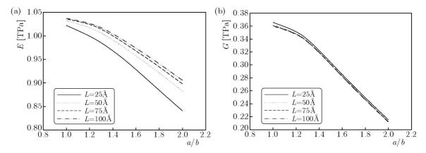
Fig. 4. Variation of Young's modulus (a) and shear modulus (b) of (5,5) with the cross sectional aspect ratio (a/b) for different lengths
