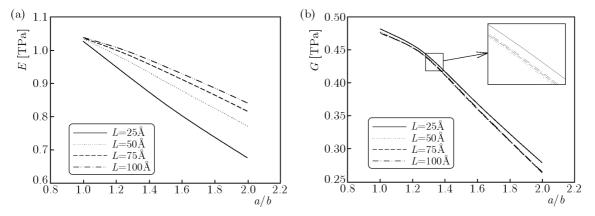
Fig. 6. Variation of Young's modulus (a) and shear modulus (b) of (15, 15) with the cross sectional aspect ratio (a/b) for different lengths
