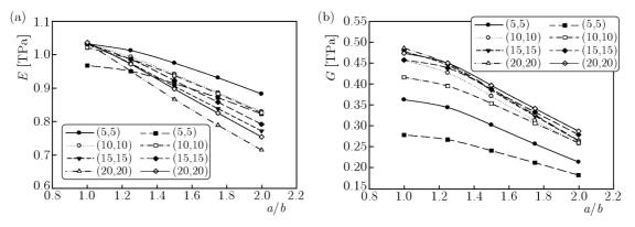
Fig. 12. Variation of Young's modulus (a) and shear modulus (b) with the cross sectional aspect ratio (a/b) and length of 50 Å
