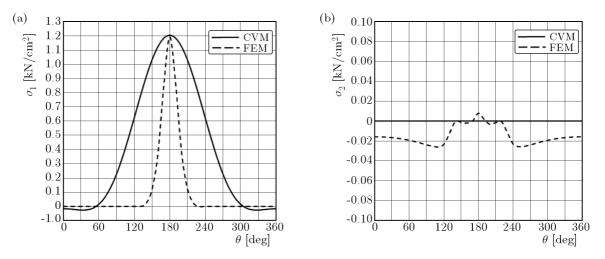
Fig. 7. Comparative diagram of the stress  $\sigma_1$  (a) and  $\sigma_2$  (b) at the outer contour of the disc
