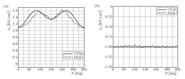
Fig. 8. Comparative diagram of the stress  $\sigma_1$  (a) and  $\sigma_2$  (b) at the contour of the eccentric hole
