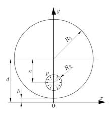
Fig. 3. The disc weakened by an eccentric circular hole
