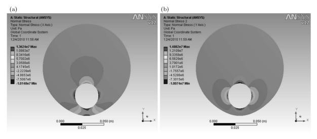
Fig. 5. Normal stress  $\sigma_x$  (a) and  $\sigma_y$  (b)
