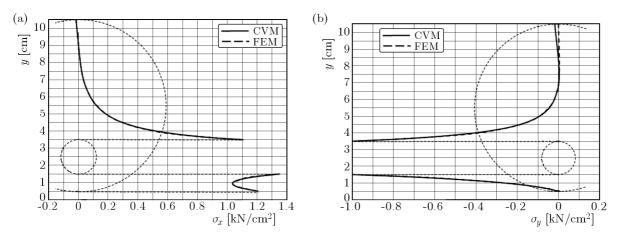
Fig. 9. Comparative diagram of the stress  $\sigma_x$  (a) and  $\sigma_y$  (b) at the intersection of the y axis
