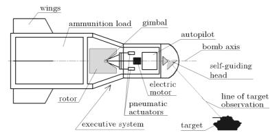
Fig. 1. General diagram of elements of the proposed guided bomb
