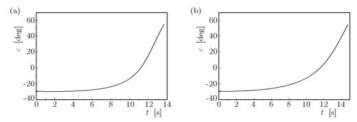
Fig. 9. Angle of inclination of the line of target observation at  $V_c = 30 \text{ m/s}$  (a) and  $V_c = 0 \text{ m/s}$  (b)
