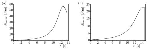
Fig. 5. Values of the controlling moment guiding the bomb on the target at  $V_c = 30 \text{ m/s}$  (a) and  $V_c = 0 \text{ m/s}$  (b)
