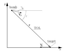
Fig. 2. Diagram of kinematics of the bomb self-guiding on the ground target
