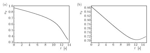
Fig. 8. Lateral overload of the bomb at  $V_c = 30 \text{ m/s}$  (a) and  $V_c = 0 \text{ m/s}$  (b)
