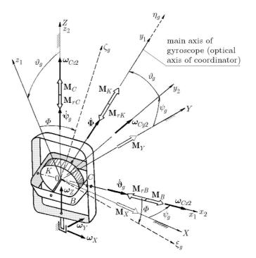
Fig. 3. Symbols used in the theory of gyroscope (Koruba, 2001, 2003; Magnus, 1971)
