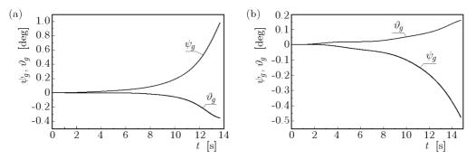
Fig. 7. Angles of deflection of the gyroscope axis (heavy rotor) necessary to the guiding the bomb at  $V_c = 30 \text{ m/s}$  (a) and  $V_c = 0 \text{ m/s}$  (b)
