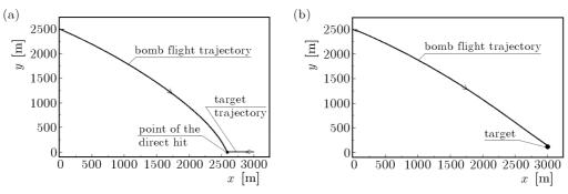
Fig. 4. (a) Bomb flight trajectory and target trajectory at  $V_c = 30 \text{ m/s}$ ; (b) bomb flight trajectory at  $V_c = 0 \text{ m/s}$
