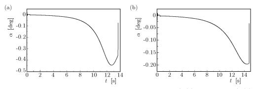
Fig. 6. Angle of attack during the bomb flight at  $V_c = 30 \text{ m/s}$  (a) and  $V_c = 0 \text{ m/s}$  (b)
