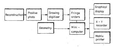
Fig. 3. The main blocks of evaluation procedure
