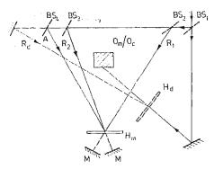
Fig. 4. Experimental setup for difference hologram interferometry
