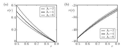
Fig. 3. Profiles of the velocity v(r,t) and the shear stress  $\tau(r,t)$  given by Eqs. (3.12) and (3.16), for  $R_1 = 0.5$ ,  $R_2 = 0.9$ , f = -5,  $\nu = 0.0357541$ ,  $\mu = 32$ ,  $\lambda = 7$ , t = 15 s, and different values of  $\lambda_r$
