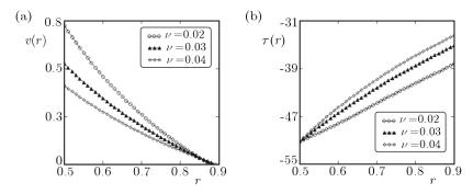
Fig. 4. Profiles of the velocity v(r,t) and the shear stress  $\tau(r,t)$  given by Eqs. (3.12) and (3.16), for for  $R_1 = 0.5$ ,  $R_2 = 0.9$ , f = -5,  $\rho = 895$ ,  $\lambda = 5$ ,  $\lambda_r = 3$ , t = 15 s, and different values of  $\nu$
