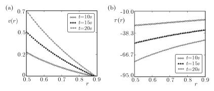
Fig. 1. Profiles of the velocity v(r,t) and the shear stress  $\tau(r,t)$  given by Eqs. (3.12) and (3.16), for  $R_1 = 0.5, R_2 = 0.9, f = -5, \nu = 0.0357541, \mu = 32, \lambda = 5, \lambda_r = 3$  and different values of t
