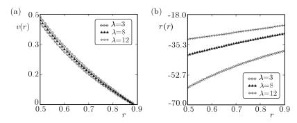
Fig. 2. Profiles of the velocity v(r,t) and the shear stress  $\tau(r,t)$  given by Eqs. (3.12) and (3.16), for  $R_1 = 0.5$ ,  $R_2 = 0.9$ , f = -5,  $\nu = 0.0357541$ ,  $\mu = 32$ ,  $\lambda_r = 3$ , t = 15 s, and different values of  $\lambda$
