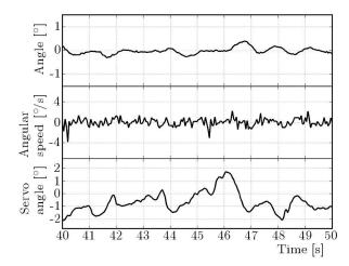
Fig. 13. Time courses of the tilt angle, tilt angular speed and servomechanism angle split into separate graphs
