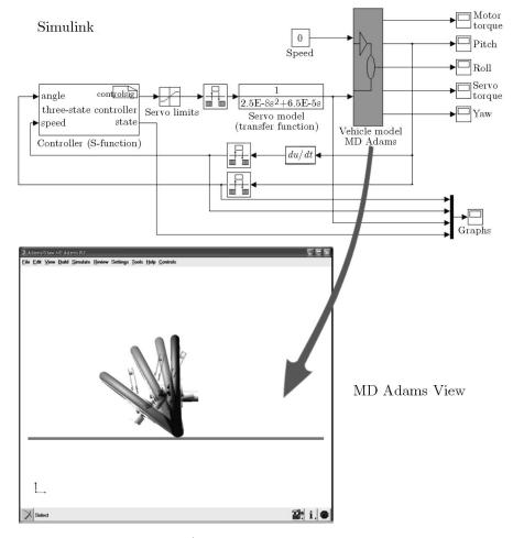
Fig. 7. The coupled Matlab/Simulink and MD Adams simulation of the robot dynamics
