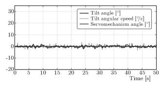
Fig. 12. Time courses of the tilt angle, tilt angular speed and servomechanism angle presented in the common graph for the test rig without disturbances
