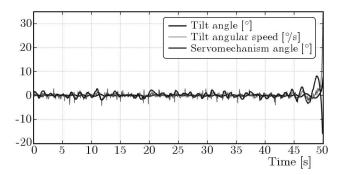
Fig. 10. Time courses of the tilt angle, tilt angular speed and servomechanism angle presented in the common graph for a test rig with a force greater than the critical
