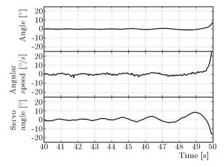
Fig. 11. Time courses of the tilt angle, tilt angular speed and servomechanism angle split into separate graphs
