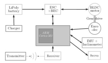
Fig. 5. The scheme of the electro-mechanical system
