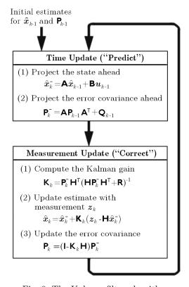
Fig. 9. The Kalman filter algorithm
