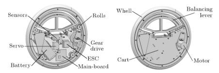
Fig. 3. The mechanical construction of the single-wheel robot
