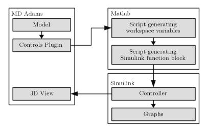
Fig. 6. The scheme of the simulation procedure
