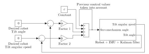
Fig. 8. Block diagram of the robot controller formula - stabilisation in the lateral plane
