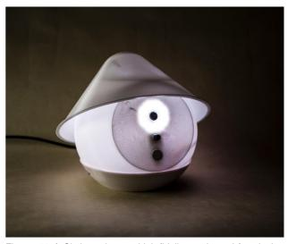
Figure 11 | Shybo robot: a high-fidelity and semi-functioning prototype.
