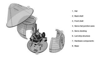
Figure 10 | 3D model of the robot's components.
