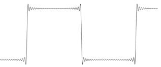
Figure 7 | Gibbs phenomenon, showing over- and undershoot, as abrupt changes undergo a sinc interpolation.
