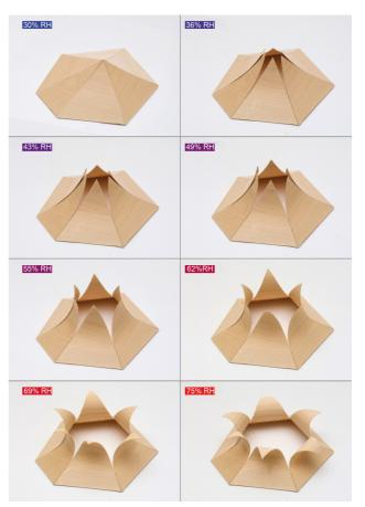
Figure 7 | HygroSkin-Meteorosensitive Pavilion / Achim Menges Architect + Oliver David Krieg + Steffen Reichert. Process-Responsive Component. Courtesy of ICD University of Stuttgart.
