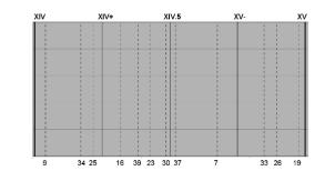
**FIGURE 2** | Virtual frets (v.fs.; solid lines) and nodes of the string up to vibrational mode 39 (dashed lines) between frets XIV and XV. Above, in roman numerals: frets/v.fs. nomenclature; below, in Arabic numerals: number of the lowest v.m. at each node.
