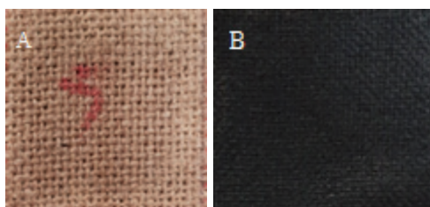
Fig. 3. Photographs of the prepared samples, A) before PDA coating and B) PDA coated fabrics.
