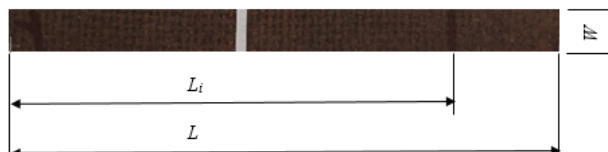
Fig. 2. Dimensions of sample used for the UL-94 testing.
