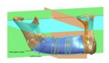
Figure 9. A shell volume model (supporting structure) together with a polygonal model of a lower jaw and the scaffold model
