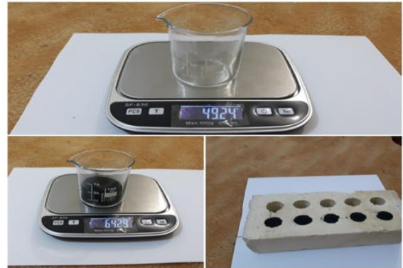
Figure 8. Put 15g of scrap tire powder into one hole
