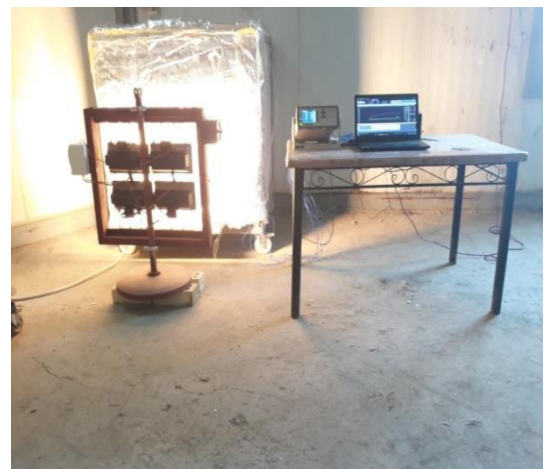
Figure 10. Apply heat source and measurement of temperatures in model No.2
