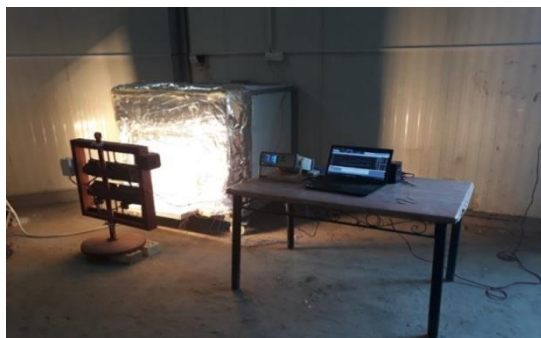
Figure 7. Apply heat source about 1200 \text{ w/m}^2 and measurement of temperatures by data logger AT4516
