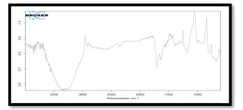
Figure 3. FTIR- Spectrum of Hydrogel of(Si-co-AA)
