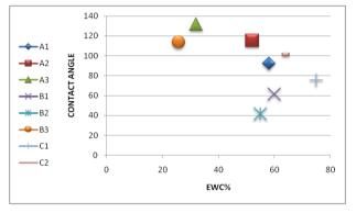
Figure 16. The correlation between EWC and contact angle for (TRIS-DMA-NVP-AA).
