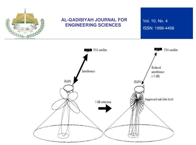
Figure 2: Main lobe and side lobes characteristic (improvement antenna radiation pattern).
