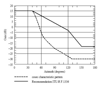
Figure 7: antenna beam pattern in azimuth direction.
