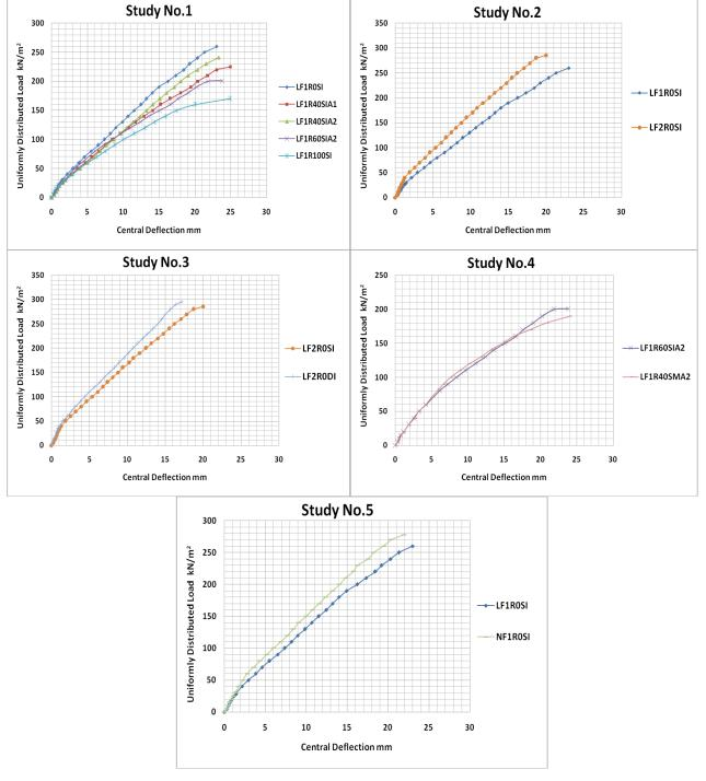
**Figure 5** Load–central deflection curve for all slab models The initial change of slope of the load-deflection curves for all slab models started between 9.47% to
