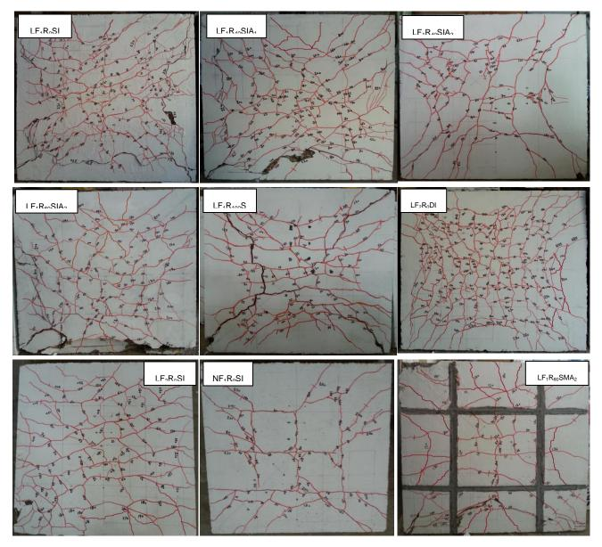
Plate 1 Cracks patterns at failure for all slab models (tension)
