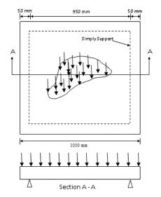
Figure 1: Details of dimensions concrete slab models.
