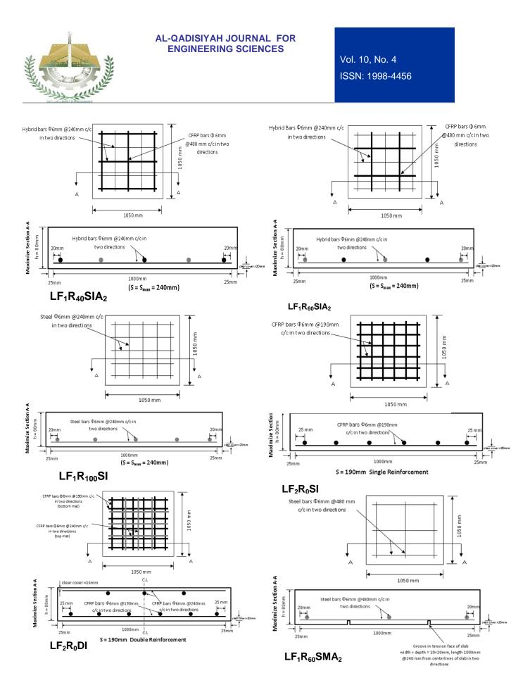
Continued of Figure 2 Details of reinforcement of slab models
