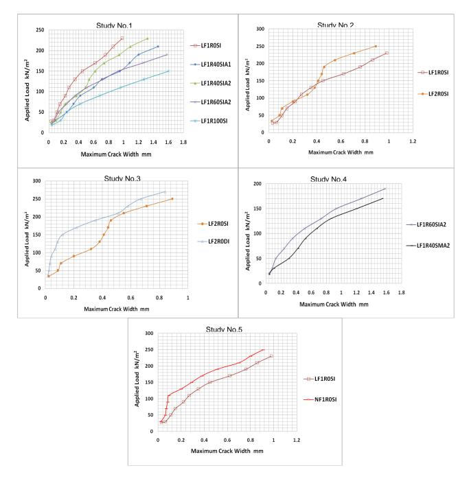
Figure 4 Maximum crack width versus load for all slab models
