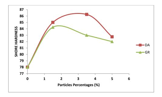
Figure (3): the relationship between the shore hardness of unsaturated polyester reinforced with grapes and dates particles
