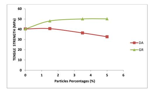
Figure (4): the relationship between the tensile strength of unsaturated polyester reinforced with grapes and dates particles
