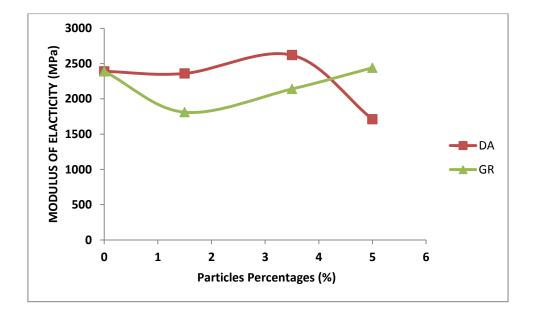
Figure (5): the relationship between modulus of elasticity of unsaturated polyester reinforced with grapes and dates particles
