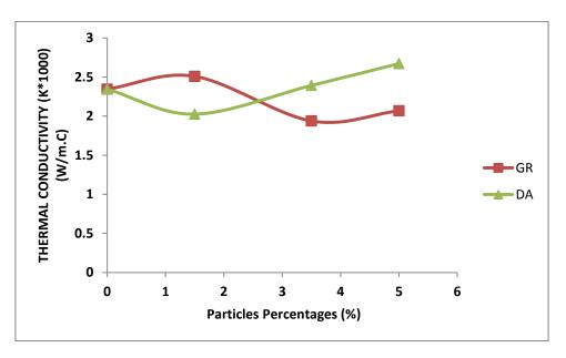
Figure (1): the relationship between the thermal conductivity of unsaturated polyester reinforced with grapes and dates particles
