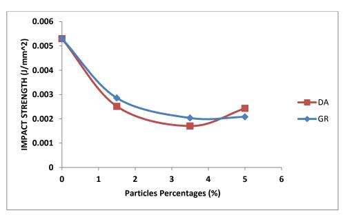
Figure (2): the relationship between the impact strength of unsaturated polyester reinforced with grapes and dates particles
