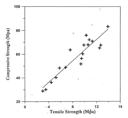
Figure (5) Shows a mathematical model for the relationship between tensile strength and compressive strength for different mixes of PMC.
